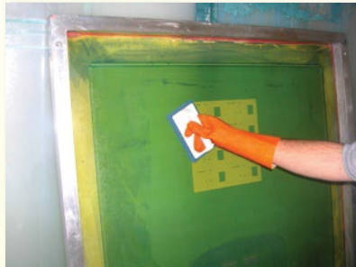
2. Scrub screen with non-abrasive pad or brush.
