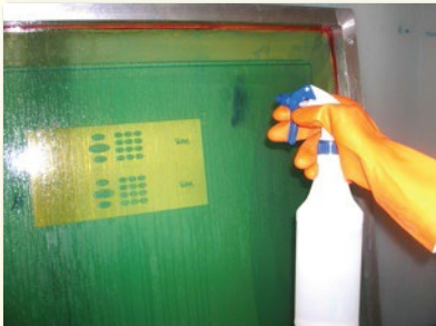
1. Spray ENVIROGRAPH on both sides of screen.
